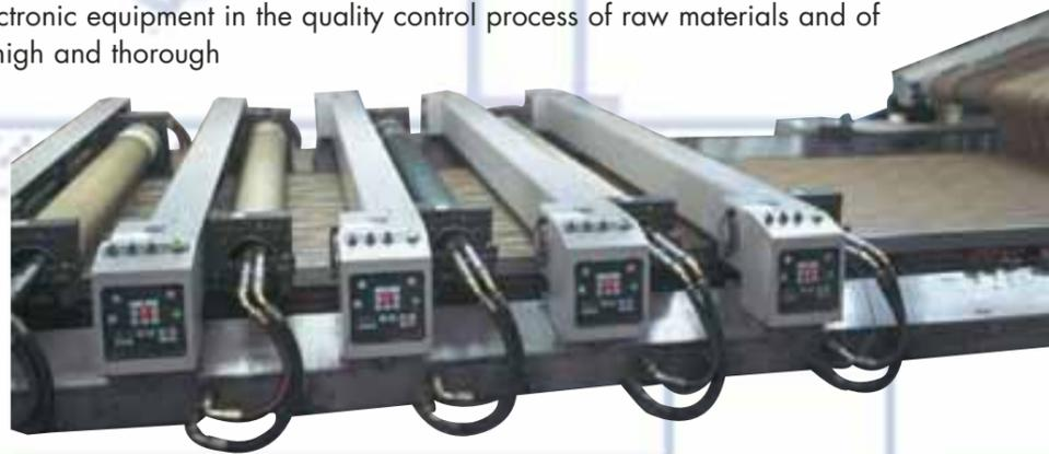
The belt has excellent resistance to oils, greases and to the chemicals normally used in the fabric printing industry, with the exception of the ketones with low molecular weight (acetone, MEK) and to the aromatic hydrogenated hydrocarbons.
